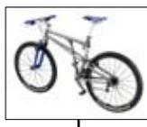
**2001** The Silk Ti was a pivotless softtail with a greater wheelbase than traditional full sus bikes. Ibis manufactured its own elastomer-sprung shock.
