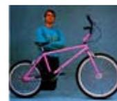
**1988** Scot's first carbon bike. It had a steel rear triangle, tapered machined lugs and carbon tubing made from the same material that Ibis use now.
