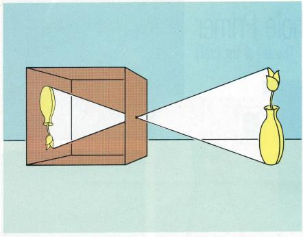
fective aperture. Forget f/64: A typical pinhole f-number can run in the hundreds—say, f/426. But if you could set such a small aperture on a lens, the lens would provide the same enormous depth of field as the pinhole—not infinite, but deep enough to eliminate the need to focus.
